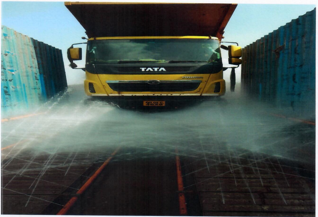
Exhibit-Water sprinkler fitted in water tanker and wheel washing system.
